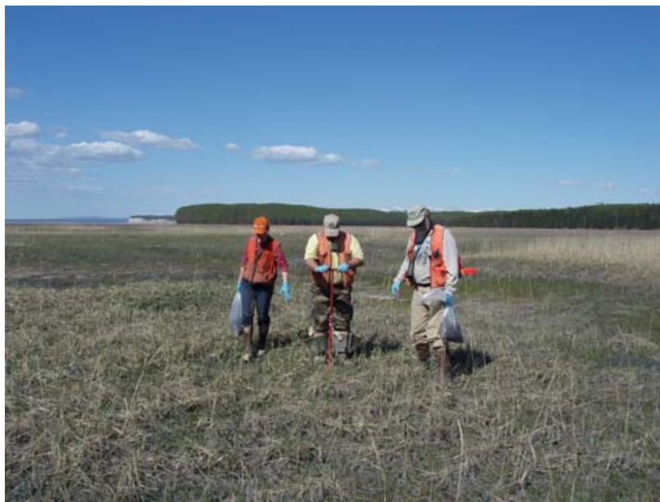
Figure 17. Field sample collection within a 30-m \times 30-m area encompassing a 120-mm mortar projectile low-order detonation. Multi-increment samples were composed of approximately 100 cores (4.75-cm ID) collected to a depth of 3 cm.
