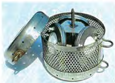
Figure 3. Commercially available stainless steel canister that will be used to house the POCIS passive samplers. The Composition B fragment will also be contained in one of these canisters and secured to pier with DoD identification tags. http://www.est-lab.com/pocis.php
