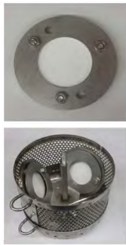
Figure 1. POCIS (top) and commercially available field holder and canister for POCIS (bottom), available from the Environmental Sampling Technologies (EST-Lab.com). Photos from Rosen et al. (2016).
