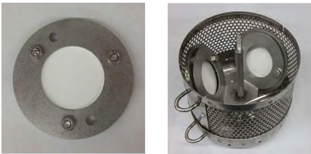
Figure 2-1. POCIS sampler (left) and commercially available field holder and canister for POCIS (right).
