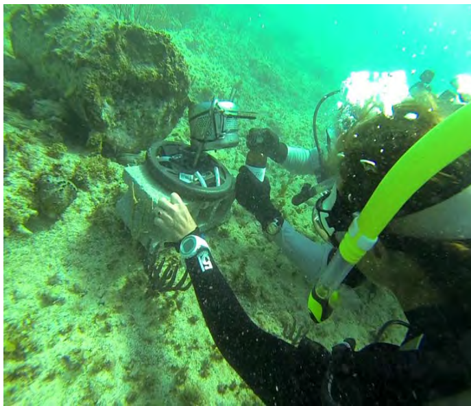
Figure 5-8. Grab sampling approach used to compare water concentrations between discrete samples and POCIS.
