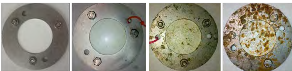
Figure 6. Examples of biofouling on POCIS after (left to right), 0, 7, 14, and 28 d of field deployment at an estuarine site (Rosen et al. 2017).
