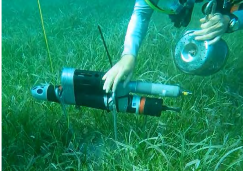
Figure 5-9. Nortek™ current profiler and Troll assembly configuration for measuring current velocity/direction and water quality adjacent to POCIS samplers. The same configuration was attached to a weighted block system at most stations for easier deployment and recovery using a lift bag.
