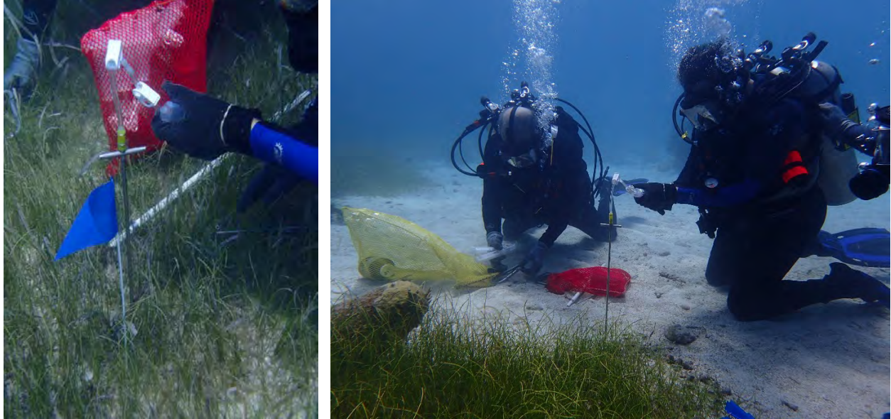
Figure 5-12. (left) Close-up of porewater sampling using PushPoint sampler, targeting top 6” sediment layer; (right) Inner station (~ 0.5 m from munition at Target Location T12) porewater sampling.
