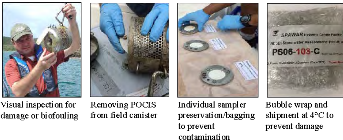
Figure 7. Upon recovery, samplers are inspected for damage and biofouling, carefully removed from the field canister, photo-documented, and individually wrapped in labeled Ziploc bags. Prior to shipment, each bag is wrapped in bubble wrap to minimize risk of membrane damage during transport.
