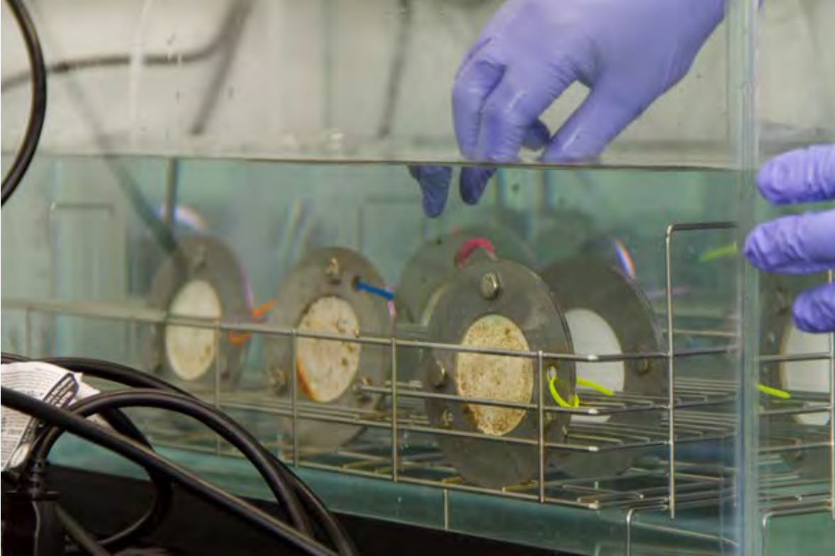
Figure B-7. Example laboratory tank showing one replicate from each field exposed time point (0 to 28 day) for POCIS prior to placement in lab exposure with nominal 1 µg/L 2,4-DNT, 2,4,6-TNT, and RDX in reconstituted seawater.
