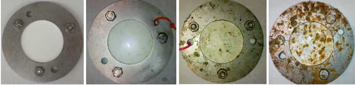
Figure B-5. Representative pictures of POCIS membranes upon initiation of 7-day MC spike laboratory experiment following deployment at Gulf Breeze East Dock (from left to right), for 0, 7, 14, and 28 days during July 7–August 4, 2015.
