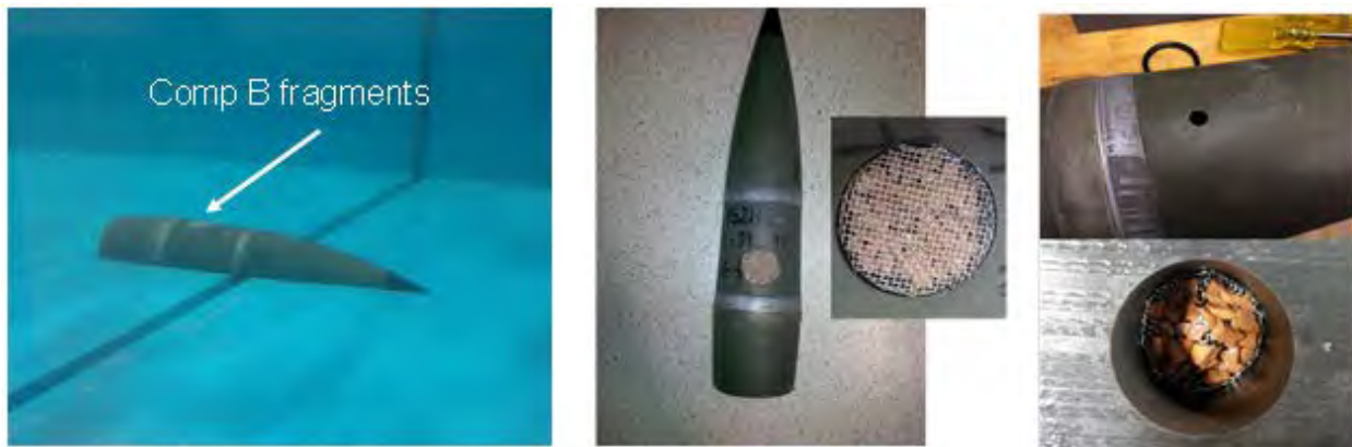
Figure 2-9. Cleaved munition surrogate produced from intact full-surrogate 155-mm replica loaded with Comp B fragments as an open source (left and center) and encased within a 1-cm hole (right).
