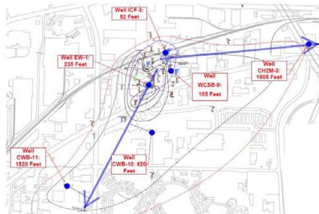
**Figure 1:** Schematic of modeled contaminant source and transport path line, and calibration wells. Wells EW-1, CWB-10 and CWB-11 were used to calibrate the south-pointing path line, while wells ICF-3, WCSB and CH2M-3 were used to verify the calibrated model as applied to the eastern-pointing path line.
