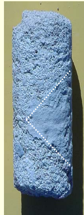
Low permeability layer in a soil core from F.E. Warren AFB
