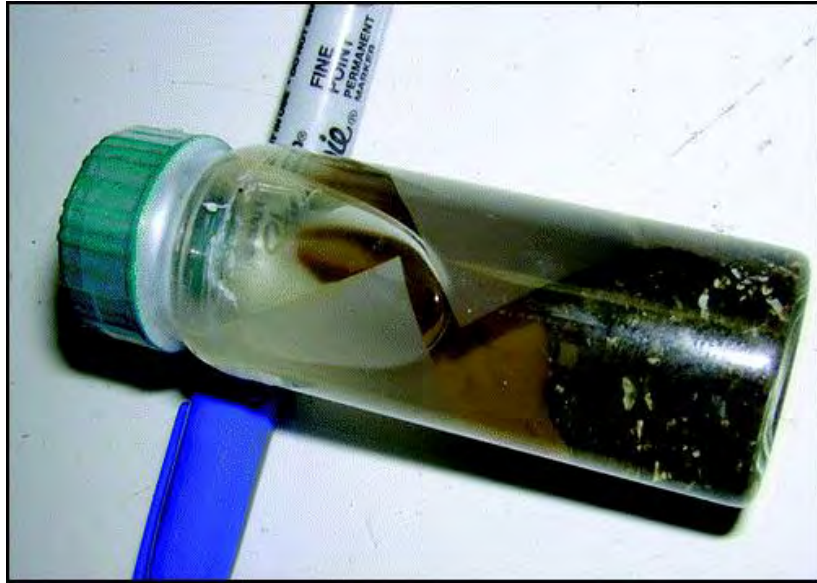
Figure 2-1. Polyoxymethylene passive sampler strip in a laboratory vial (40 mL) for an ex situ deployment in a water-sediment slurry for sampling interstitial waters (image provided by SB Hawthorne [University of North Dakota, Grand Forks, ND, USA]).
