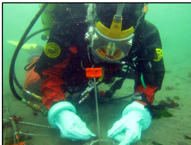
Figure F-8. U.S. EPA scientific diver Brent Richmond places a SPME passive sampler at the Wyckoff Superfund Site (image by Sean Sheldrake).
