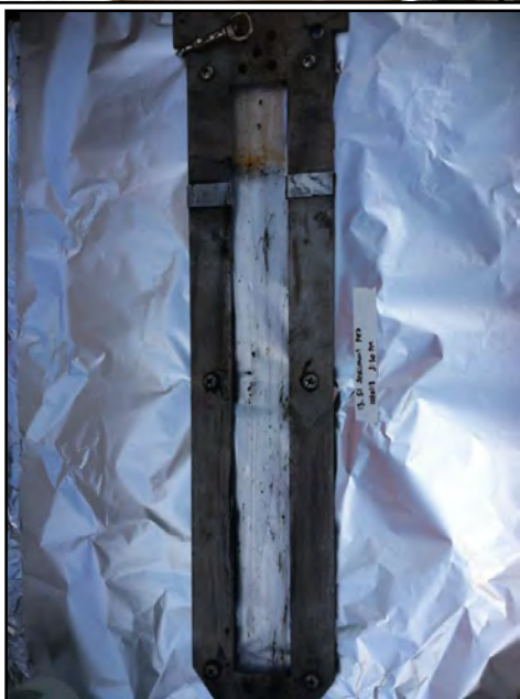
Figure F-10. Assembly of samplers prior to deployment (top), and a sampler after retrieval (bottom), showing the sediment/water interface right above the white tape mark. The total length of the LDPE window was ~50 cm.
