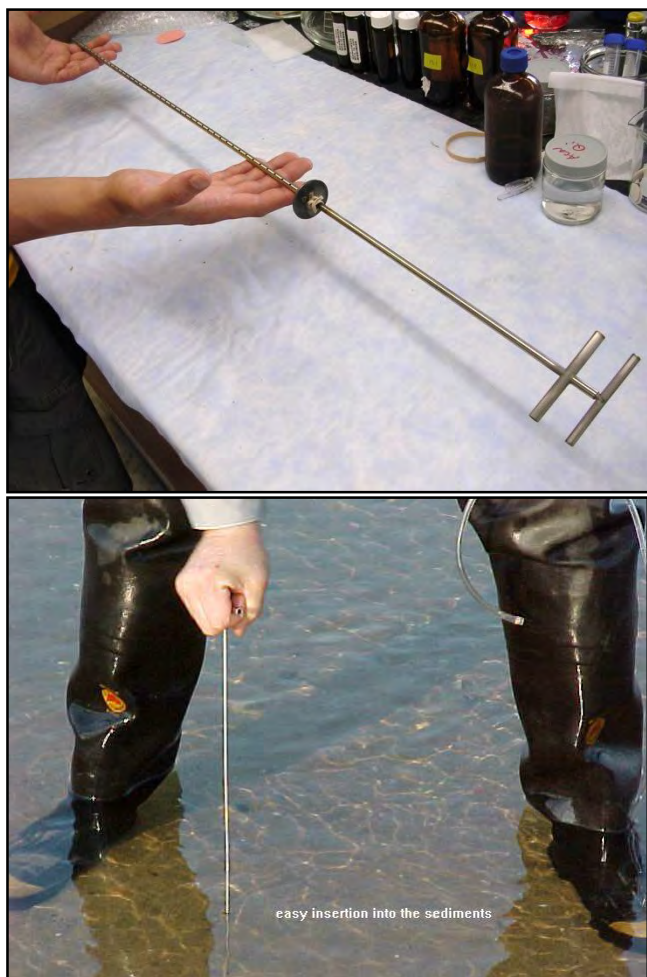
Figure F-4. SPME sampler in the laboratory (upper) and insertion into intertidal sediment in the field (lower) (figures from Reible and Lu (2011)).
