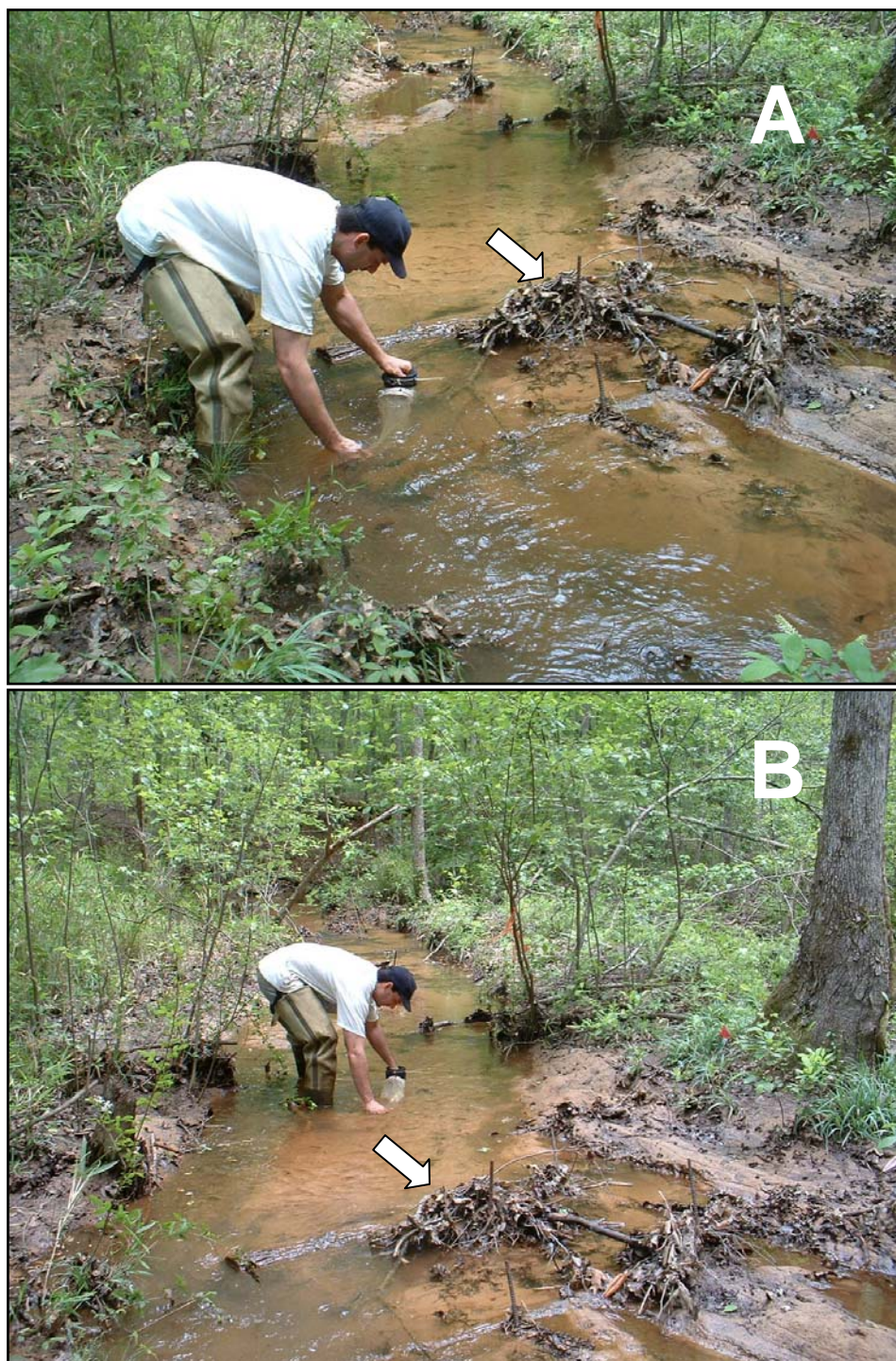
Figure 80. Photographs showing T-sampling of benthic macroinvertebrates inside (A) and outside (>3m upstream) (B) of artificial debris dam additions. This approach was used to quantify microhabitat-specific differences in macroinvertebrates assemblages, streambed benthic particulate organic matter accumulation (BPOM, Fig. 81), and algal biomass abundance (as chlorophyll a , Fig. 91) in the stream bed attributable to instream restorations. Arrows show artificial debris dam; note accumulations of leaf litter and coarse woody debris.
