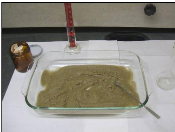
c. Final acetone–soil slurry.
