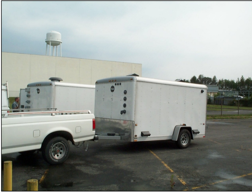
Figure 5-18. Photograph of biosparge trailer units.
