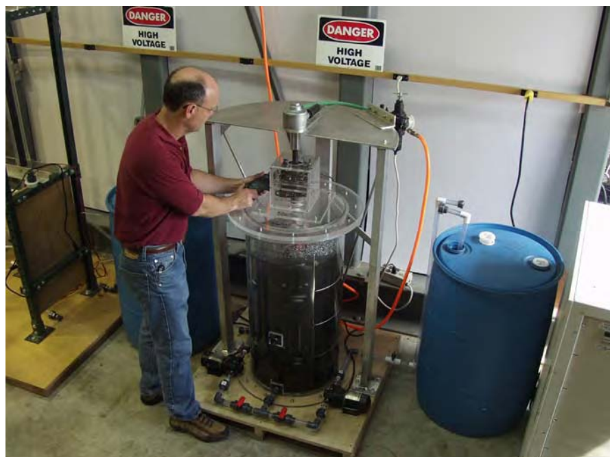
Figure 17. Rotating electrode batch reactor.
