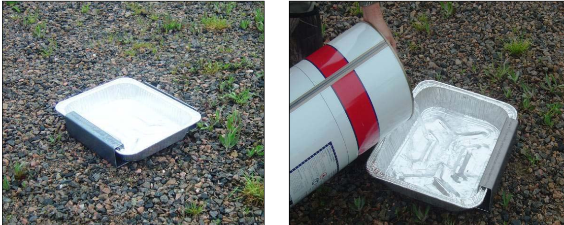
Figure 3-5. Particle trap and holder (left) being filled with ethanol (right).
