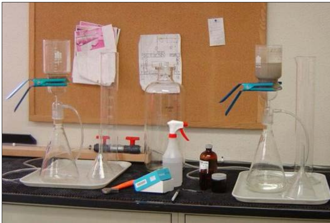
Figure 2-8. Snow sample filtration setup at the CRREL analytical laboratory.
