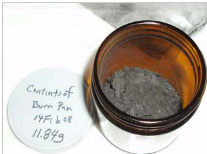
Figure 7-15. Processing of the burn bowl residues; loose residues from bowl.
