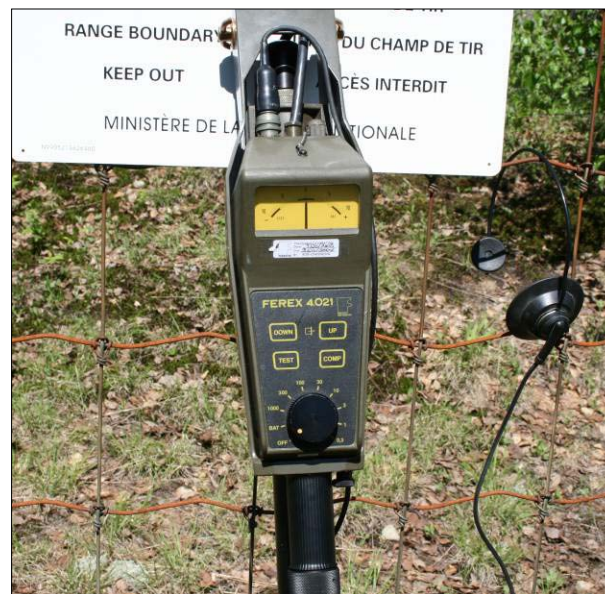
Figure 5-8. Forester metal detector used for proofing.
