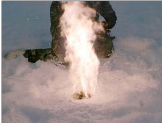
Figure 7-4. 81-mm propellant burn test on snow.
