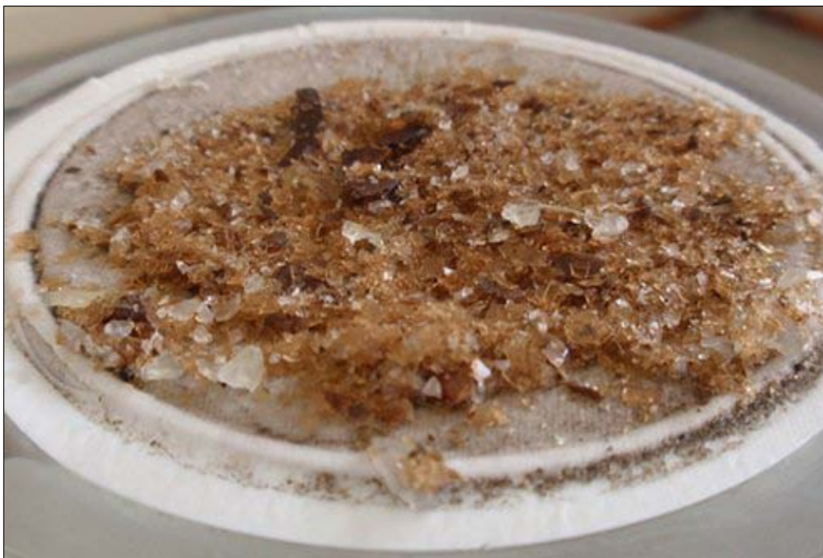
Figure 2-11. Filtered mass from back plume sample. Beige material is propellant. Filter paper is 90 mm in diameter.
