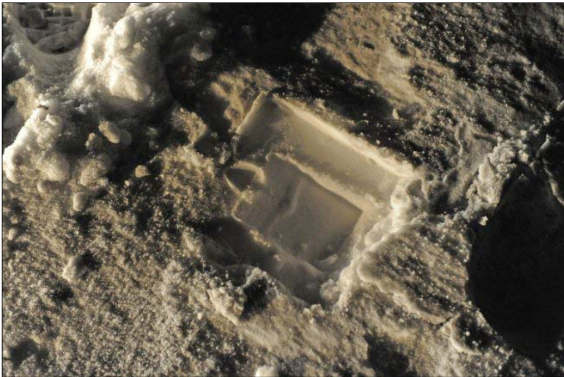
Figure 4-7. Sampling snow at the surface and below the surface.
