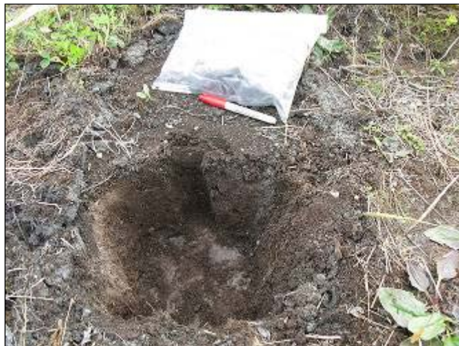
Figure 7-13. July resampling of 120-mm mortar propellant burn sites, showing depth samples.
