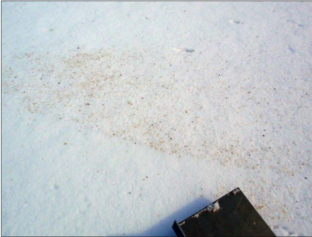
Figure 2-7. Propellant debris on snow in back plume following rocket firing. Edge of scoop is 10 cm long.
