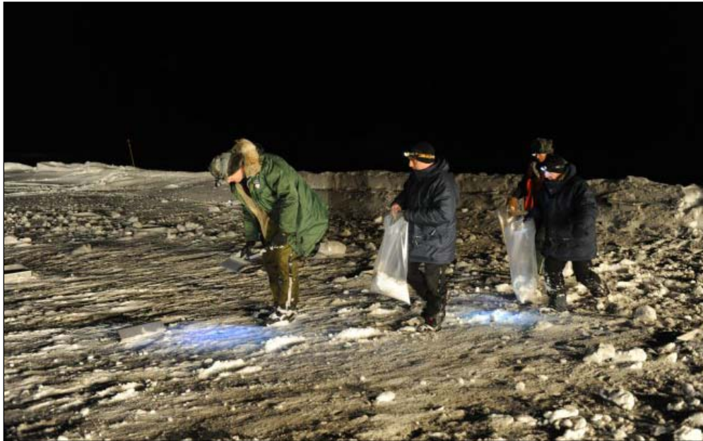
Figure 4-19. Sampling snow using 20- x 20-cm scoop.
