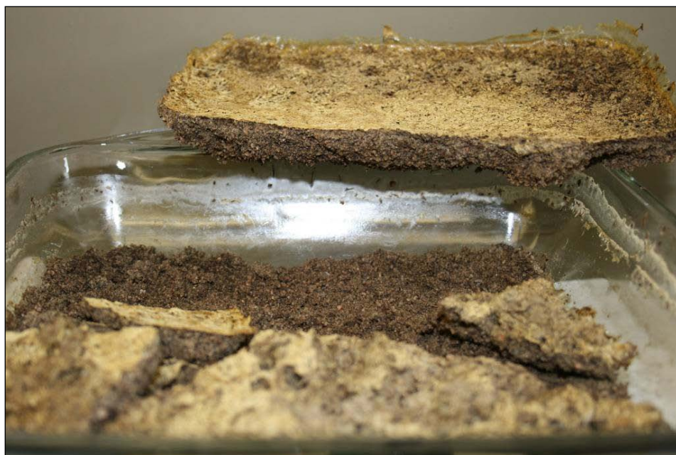
Figure 5-17. Carpiquet surface soil sample S-Car-Rep-1 after acetone homogenization.
