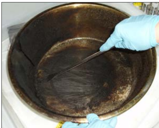
Figure 7-16. Cleaning the char from the burn bowl.
