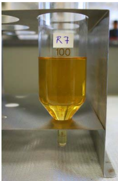
Figure 4-22. Acetonitrile extraction of the pails.
