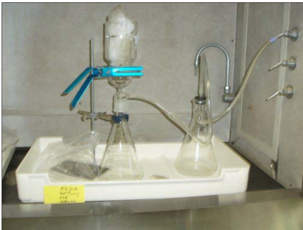
Figure 2-10. Setup at CRREL's laboratory for filtering propellant debris from March snow sample.
