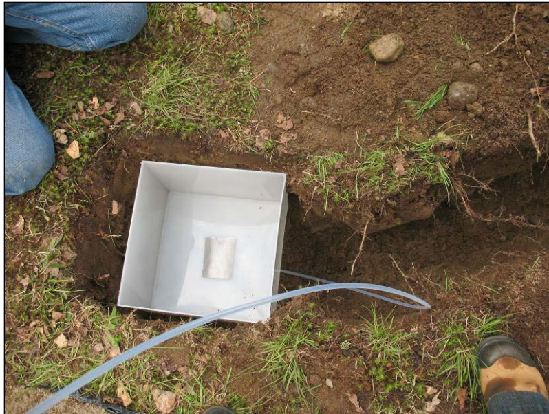
Figure 5-11. Installation of lysimeters at Carpiquet.
