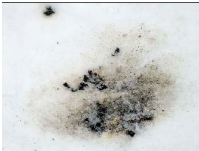
Figure 7-5. 81-mm propellant burn residues.
