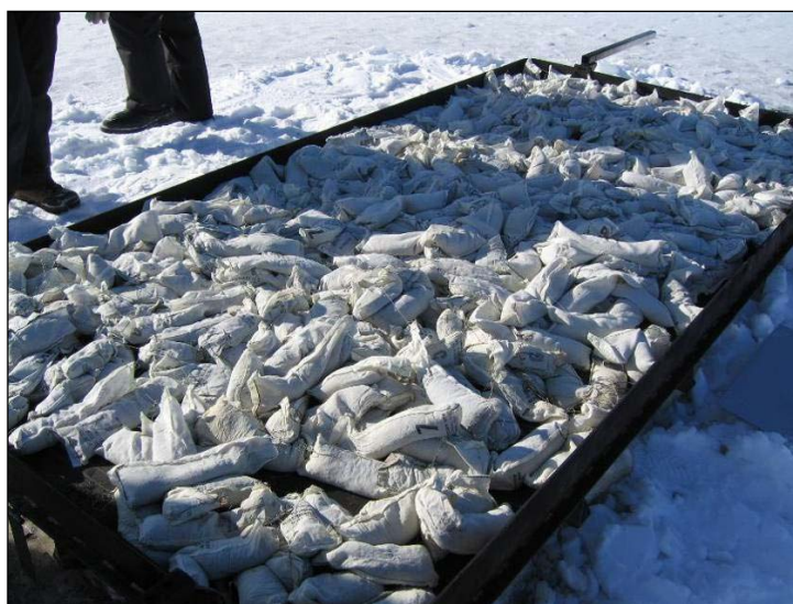
Figure 8-19. Gun propellant bags on table before ignition.
