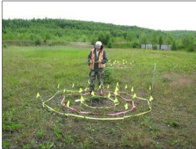
Figure 7-12. July resampling of 120-mm mortar prop burn sites, showing sampling areas.
