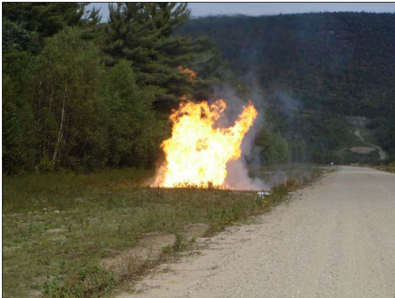
Figure 8-13. Burning of gun propellant lines.
