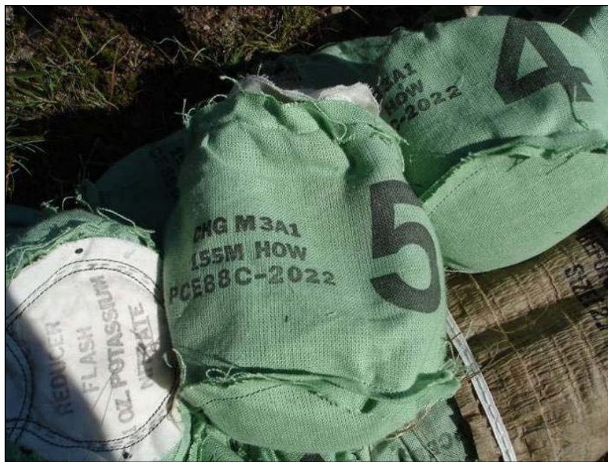
Figure 8-4. Gun propellant bags: M3A1, 155-mm caliber.
