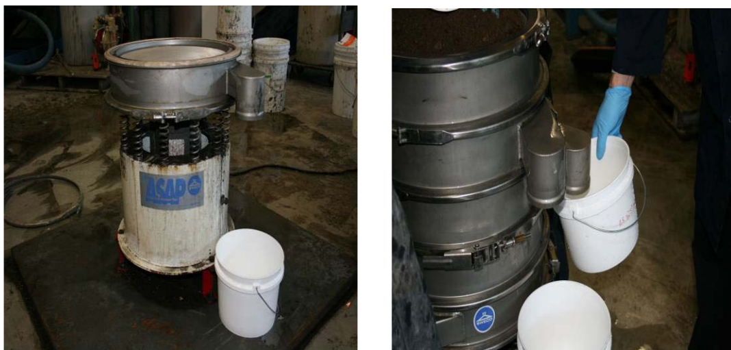
Figure 5-18. Sample sieving at INRS-ETE laboratory for the DRDC sample.
