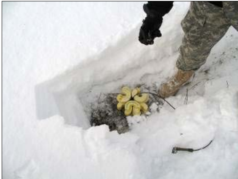
Figure 7-7. 120-mm propellant burn tests, charges on frozen soil.
