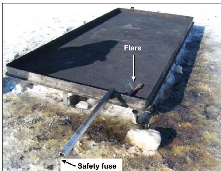
Figure 8-18. The flare in one corner of table.
