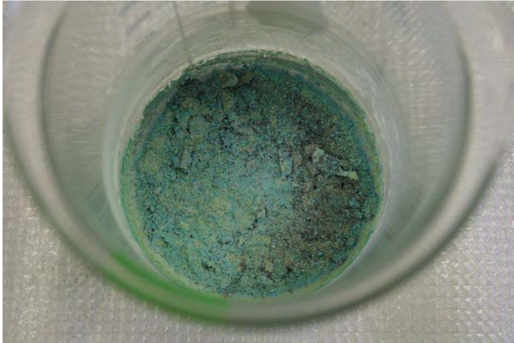
Figure 4-24. Green solid isolated by evaporation.
