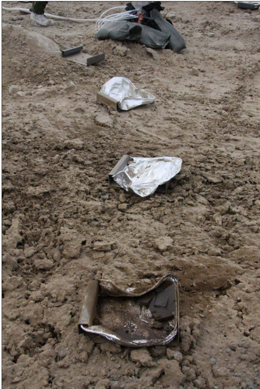
Figure 4-3. Particle traps destroyed during November 2008 trial.
