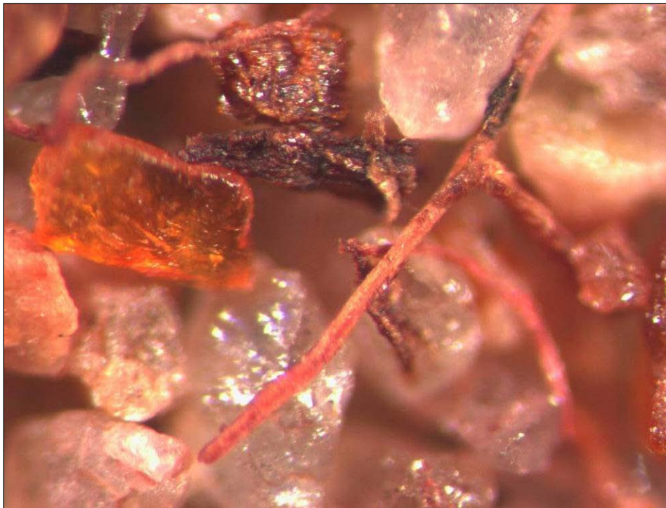
Figure 5-26. A sieved soil fraction between 1 and 2 mm.
