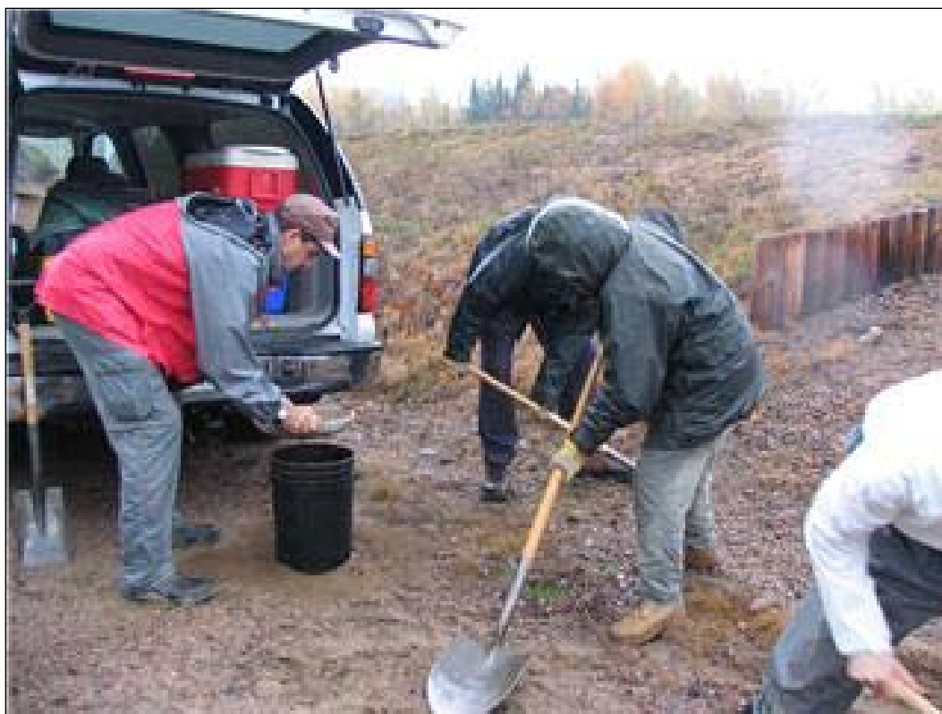
Figure 6-3. Sampling of propellant residues at the firing positions on antitank training range A, at CFB Petawawa.
