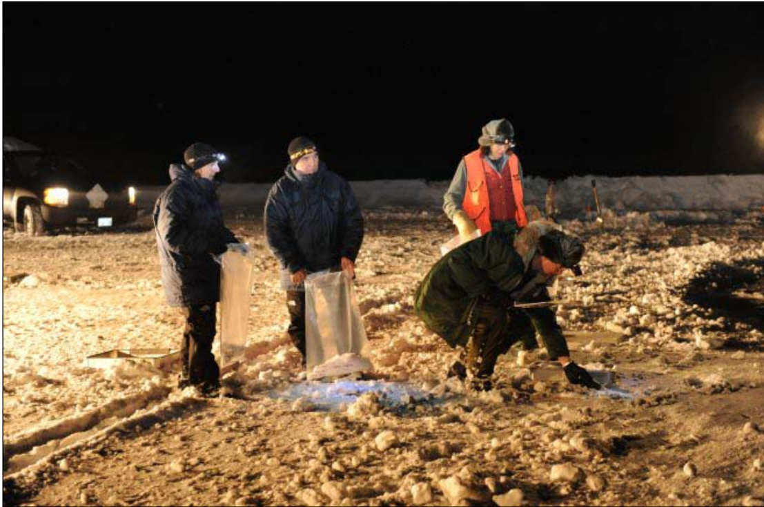
Figure 4-6. Collecting particles using the snow collection method.
