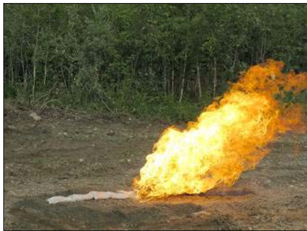
b. Propellant burning on wet sand.
