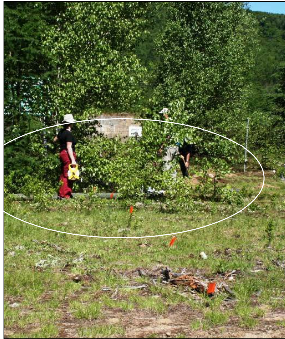
Figure 5-5. Sampling DU-C to DU-H. The flags delineate the limits of each DU.
