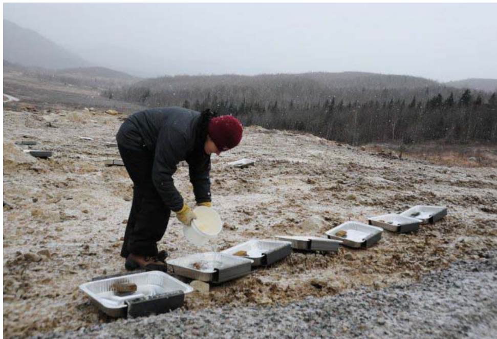
Figure 4-14. Particle traps in holders with weights.
