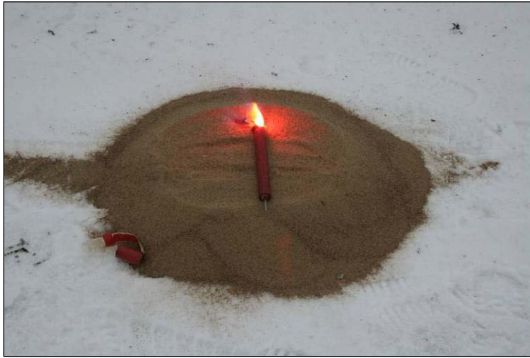
Figure 8-16. Setup for flare trial (part for the flare only: Line #3).
