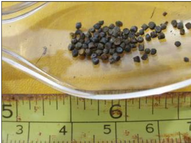
c) June 2008 recovered unburned propellant.
