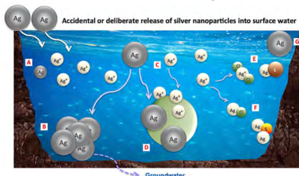
Figure 1 Possible fates of silver nanoparticles in surface waters: (A) Dissolution process leading to free ions release and smaller particles; (B) Aggregation into larger particles, which may settle out of the water, depending on the aggregate size; (C, D) Adsorption of released Ag^+ and nAg , respectively, onto other solids present in the water; (E) Formation of soluble complexes; (F) Reaction with other components in the water, which may result in precipitation; (G) nAg remaining stable.
