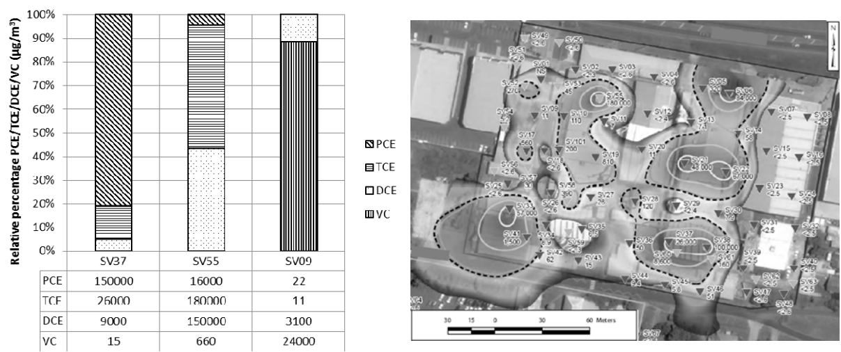
Fig. 1. Typical PCE (SV37), TCE/DCE (SV55) and VC dominant SV results, indicating variability in contaminant type/degradation; and example isopleth plot for TCE in SV across the Site (dotted line represents adopted criterion, units in \mu\text{g}/\text{m}^3 ) (after SiREM 2015)
