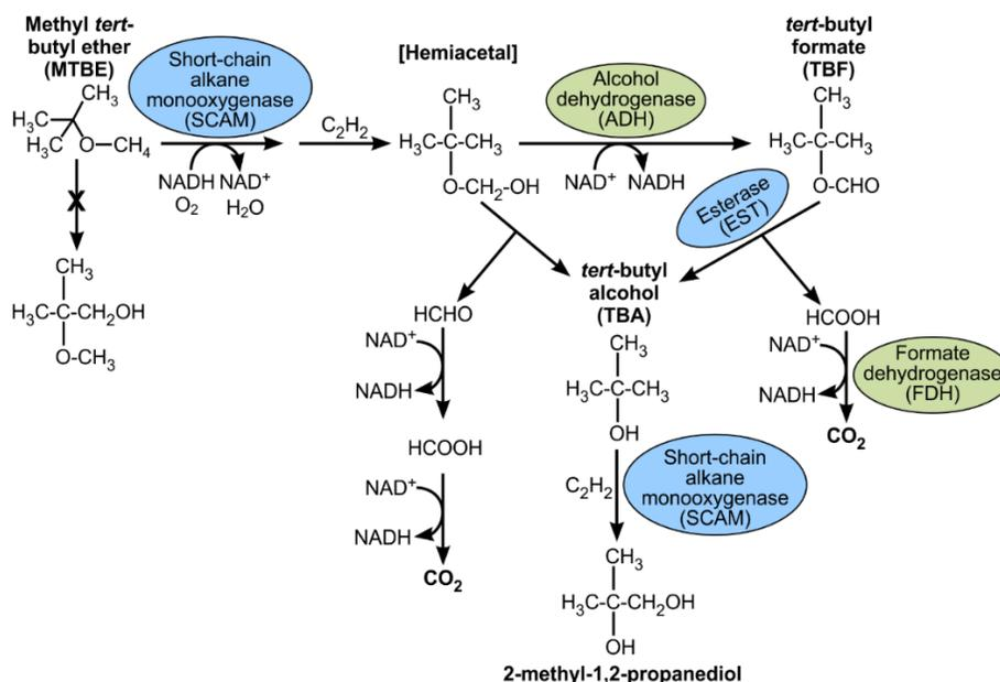
**Figure 2.0-2. Initial Reactions and Corresponding Enzymes Determined in Cometabolic Degradation of MTBE by Propane-Grown *Mycobacterium austroafricanum* JOB (Smith, O'Reilly et al. 2003; Nava, Morales et al. 2007)**
