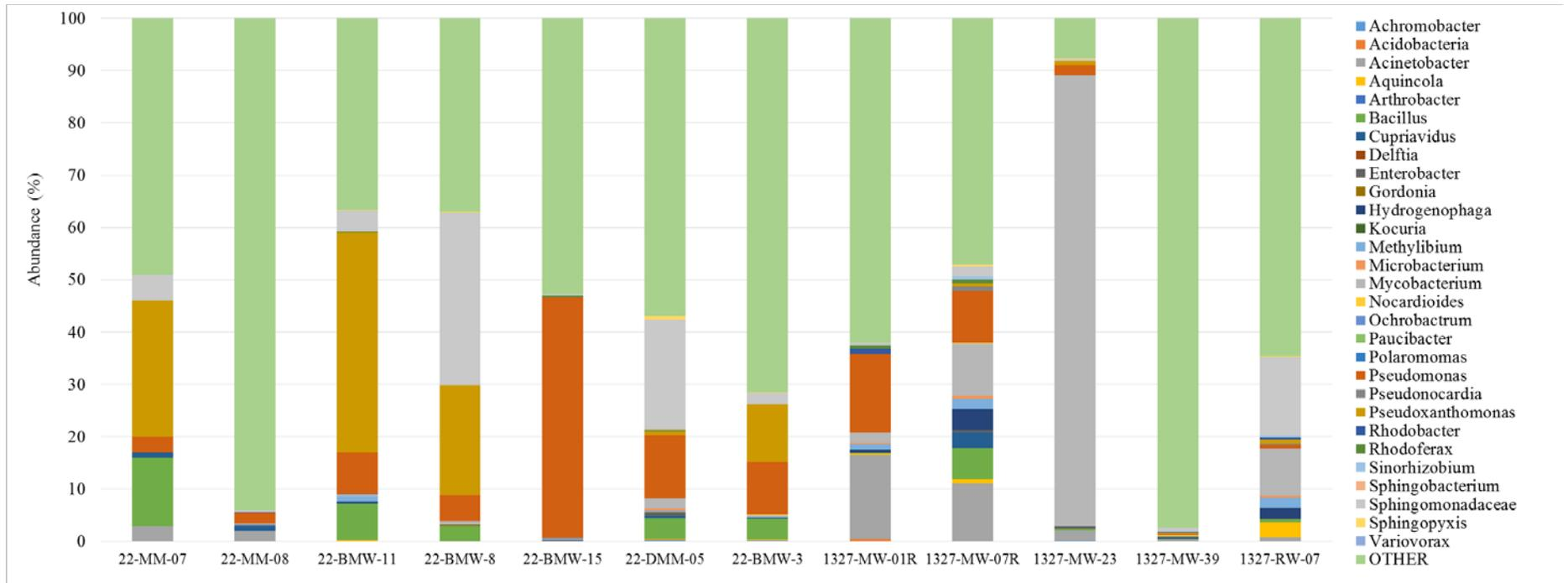
**Figure D-18. Percentage Abundance of Microbial MTBE and TBA Degrading Microorganisms on Genus Level Detected in Samples Collected from 22 Area MCX Gas Station and 13 Area Camp Pendleton Site during Sampling Event 2**
