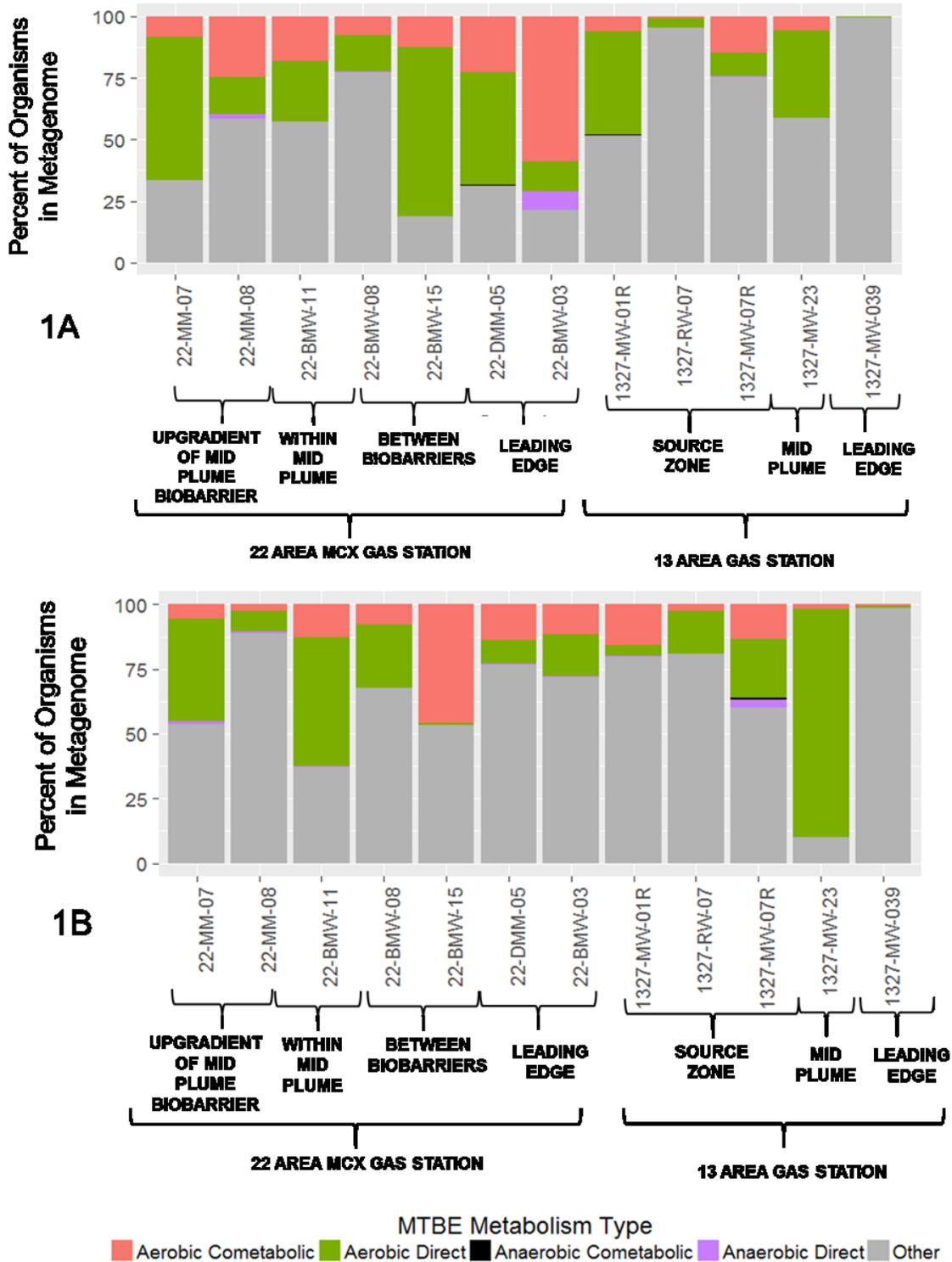
**Figure 5-4. Percent Abundance of Microorganisms in Samples from the 22 Area MCX Gas Station and the 13 Area Gas Station where 1A is the First Sampling Event and 1B is the Second Sampling Event. MTBE-degrading Microorganisms were Categorized Depending on Aerobic/Anaerobic and Direct versus Cometabolic Degradation.**
