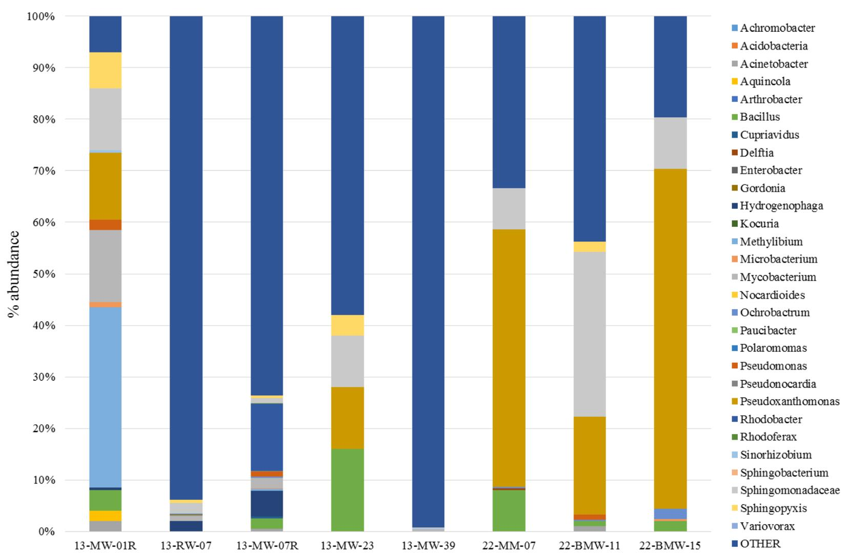
**Figure D-16. Percentage Abundance of Microbial MTBE and TBA Degrading Microorganisms on Genus Level Detected in Samples Collected from 22 Area MCX Gas Station and 13 Area Camp Pendleton Site during Optional Sampling Event**
