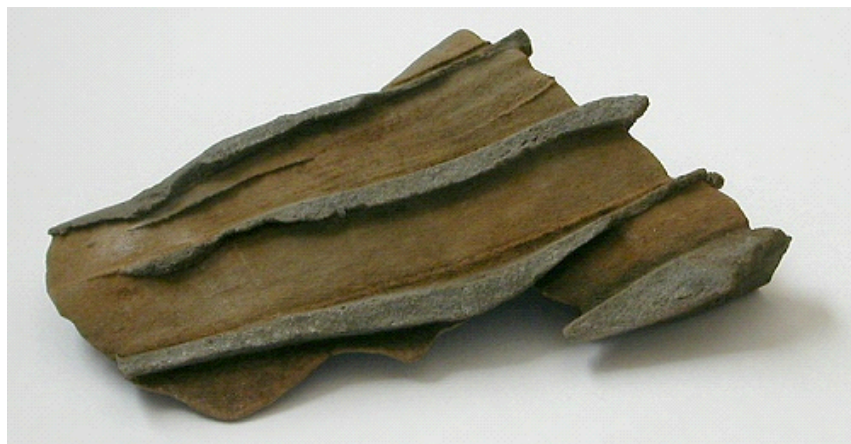
FIGURE 2-4 Interbedded sandstone and shale, shown as an example of Type III media. SOURCE: Reprinted, with permission, from http://geology.about.com . © 2004 About.com.
