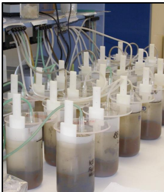
Figure 5-3. Photograph of the ex situ deployment of DGT samplers in simulated water column – whole sediment system (image provided by S Simpson [CSIRO, Sydney, Australia]).
