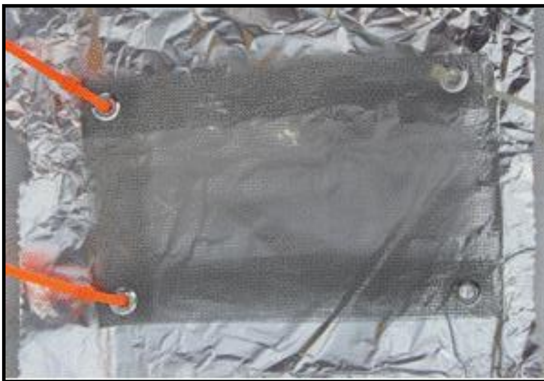
Figure 4-3. LDPE film deployed inside an aluminum mesh packet.
