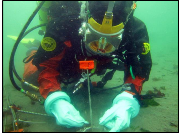
Figure F-8. U.S. EPA scientific diver Brent Richmond places a SPME passive sampler at the Wyckoff Superfund Site (image by Sean Sheldrake).
